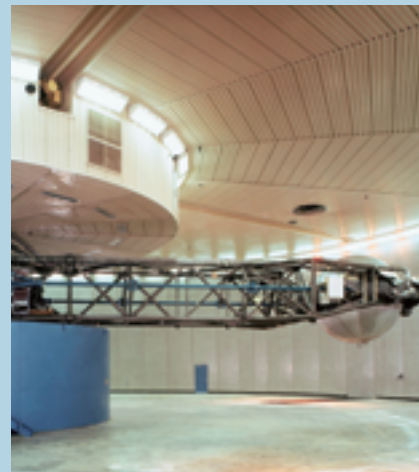
Figure fp.8 Astronauts are tested in a g-force simulator before being allowed to go on space missions. The astronaut is seated in the chamber at the end of the spinning arm.
