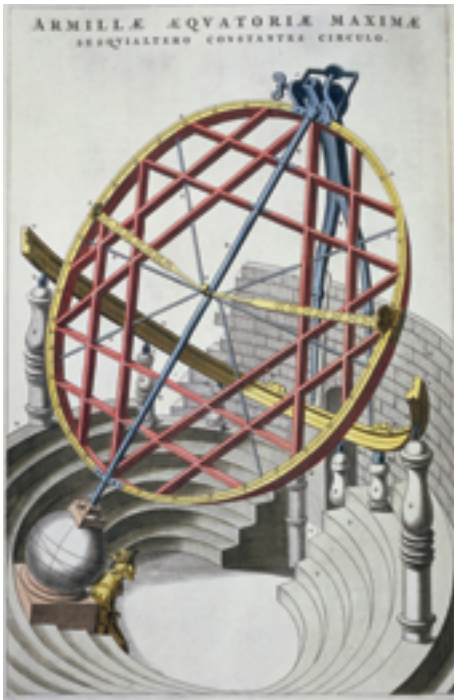
Figure 6.60 Brahe's 'Great Armillary', one of the instruments with which he measured the positions of the stars and planets.
