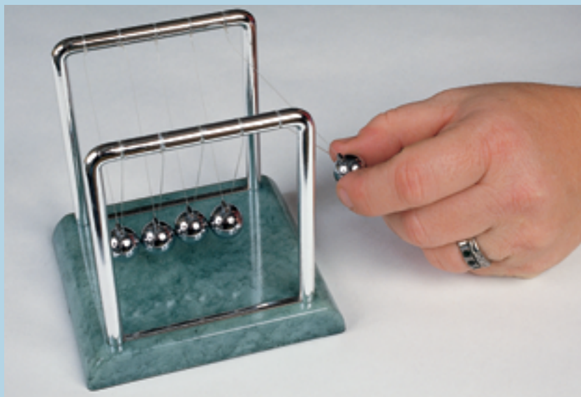
Figure sm.14 Newton's cradle is an 'executive toy' based on the principle of conservation of momentum extended over a number of objects.
